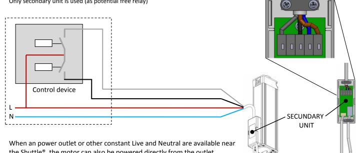
the Shuttle<sup>®</sup>, the motor can also be powered directly from the outlet. The power plug, attached to the secondary unit, can then be removed.
